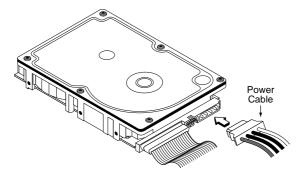
Figure 8. Connecting cables to the drive
