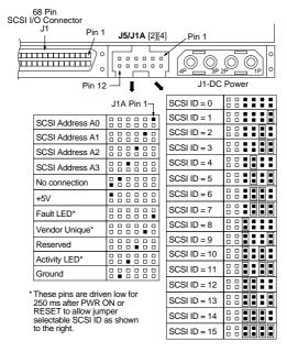
Figure 11. Alternate SCSI ID select and LED connection
