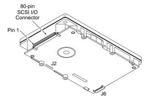
Figure 14. 80-pin I/O connection to drive
