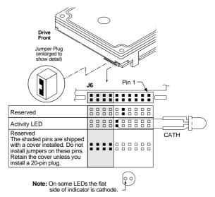
Figure 6. Drive Active LED indicator connections
