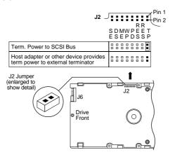
Figure 5. Setting terminator power jumpers
