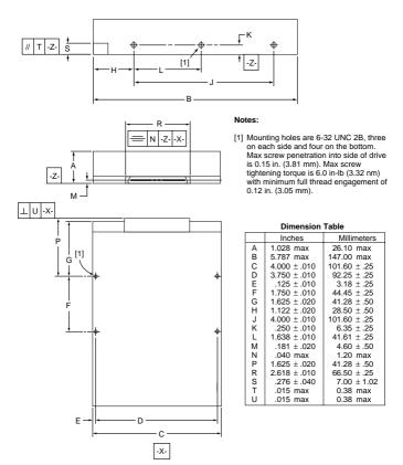
Figure 15. Mounting configuration dimensions
