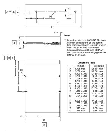
Figure 10. Mounting configuration dimensions
